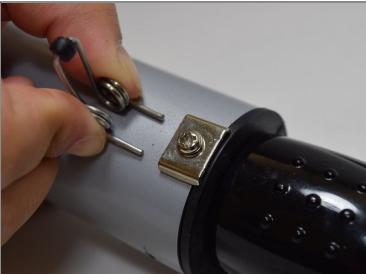
• Squeeze both sides of the barrel clip spring, and slide the component away from the barrel to remove.
