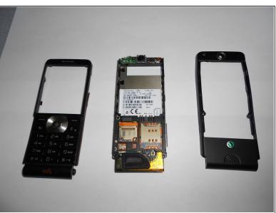
Using an opening tool and a gentle outward motion, separate the front plate from the inner phone workings.
