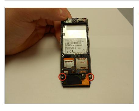
Using a T5 screwdriver, remove the two screws by turning them counterclockwise.
