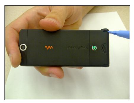
Place the plastic opening tool in the bottom corner of the phone in the crevice between the flap to remove the cover.
