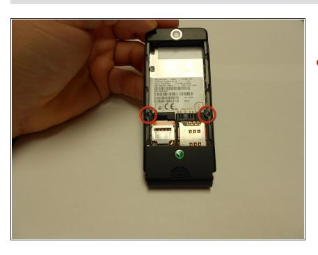
Using a mini Phillips screwdriver, remove two screws by turning them counterclockwise.
