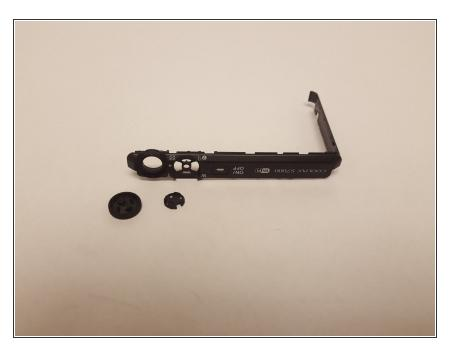
After following all previous steps and the button is still jammed or sticky, it may be necessary to replace the button. To do so follow this Button Replacement guide <u>Nikon Coolpix</u> <u>\$57000 Navigation Button</u> <u>Replacement</u>. To reassemble your device, follow these instructions in reverse order.
