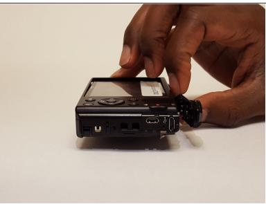
Remove outer camera frames by carefully pulling the frame apart from the body of the camera.
