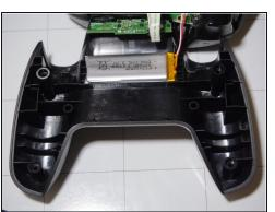
⚠ Be mindful of the three cables still connecting the two halves.
