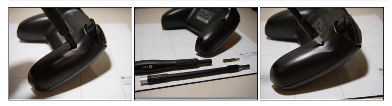
The two screws on the top are further inset than the others. You can use the iFixit 1/4" to 4 mm Driver Adapter as an extender.
