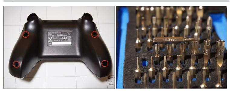
Start off by removing the four TR9 Torx Security screws on the back of the controller.
