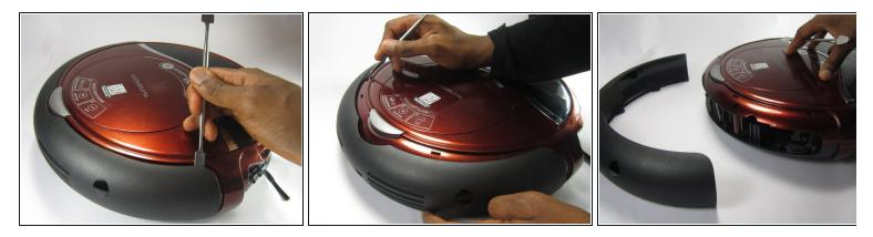
• Pry off the back bumper by going around the entire top of the bumper with the metal spudger.
