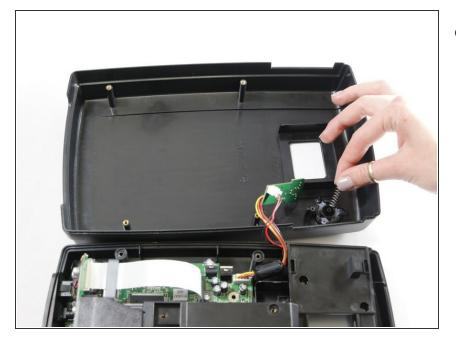
• Remove the spring and replace it with a new one.
