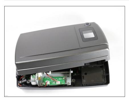
Once the screws have been removed, with light force open the scanner by pulling it apart at the seam.
