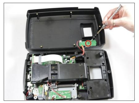
• With a JIS J0 screwdriver remove the 1 screw that is 7mm x 6mm.
