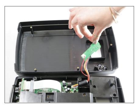
• Lift and move the plate with the connected wires out of the way.
