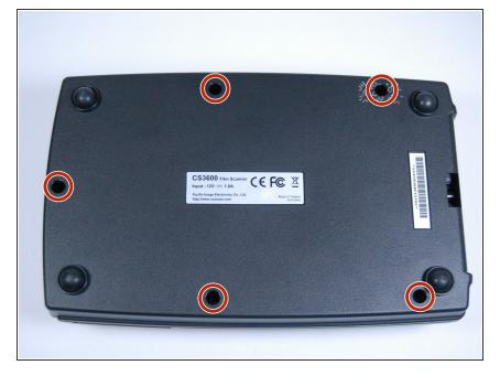
Begin opening the device by unscrewing the 5 following 9mm x 7mm screws with a J1 screwdriver.
