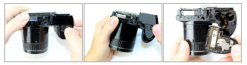
• Once the rear case is removed, gently separate the battery compartment door from its position.
