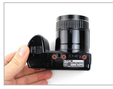
• Remove the three 5.0 mm JIS #000 screws on the bottom of the camera.
