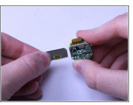
Get the GPS/Button Component by itself and use the Spudger tool to lift the silver cover off the GPS Component. This will expose the GPS Component.
