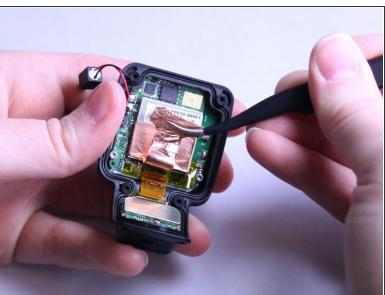
Now lift the smaller square of copper off the front panel. Use the precision tweezers and slide it under the smaller square of copper lining then gently lift it up.
