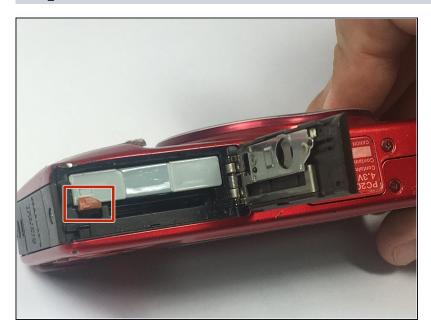
Depress the orange lever holding the battery in place to unlock it.
