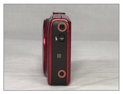
• Use a #000 Phillips screwdriver to unscrew the four 4mm screws located on the sides of the camera (2 for each side).
