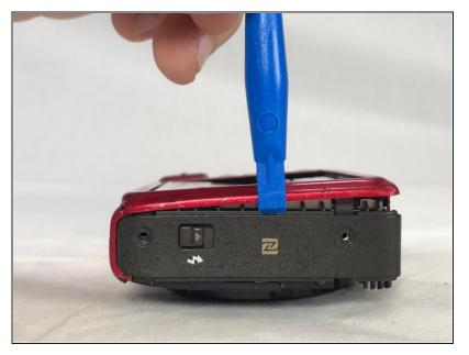
Use a plastic opening tool to loosen and remove both the front and back plates of the camera, as well as the two side pieces.
