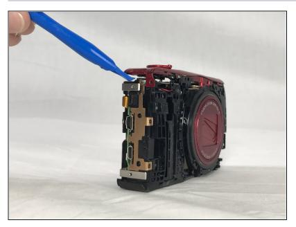
Use an opening tool to gently remove the power and shutter button assembly from the frame.
