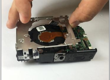
Gently remove the frame. (Make sure to have a firm hold on the rest of the camera at this point)
