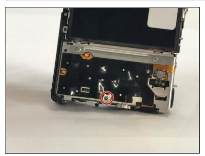
• Use a Phillips #000 screwdriver to unscrew the 4mm screw.
