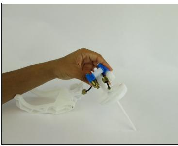
Use pliers to unscrew the gold cap piece from both ends of the tube
