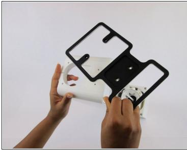
Remove the four 17.8 mm screws from the bottom metal base using a Phillips #1 screwdriver.
