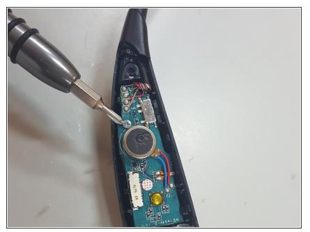
• Using a Philips #00 screwdriver remove the screw holding the motherboard in place.
