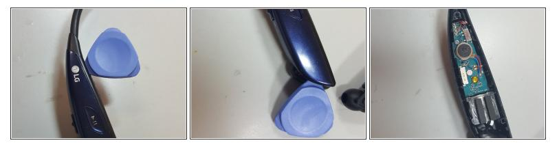
• Using a guitar pick or any opening tool, open the frame of the headset.
