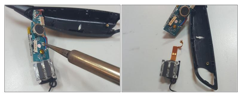
• Use a soldering iron to desolder the speaker from the motherboard.
