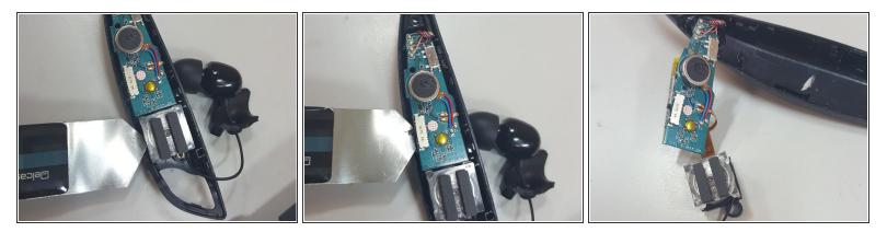
• Using a pry/opening tool, slightly lift the speaker and motherboard out of place.
