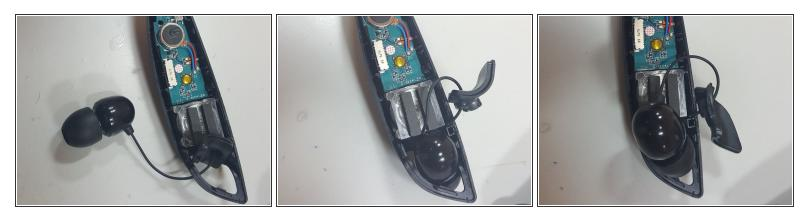
Slightly push back on the speaker back housing so the speaker can be pushed out as seen in the pictures.
