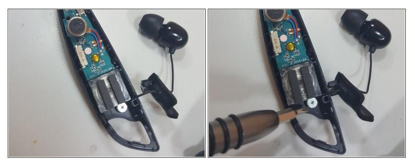
Once the speaker is out of the way, the hidden screw can be removed using a Philips #00 screwdriver.
