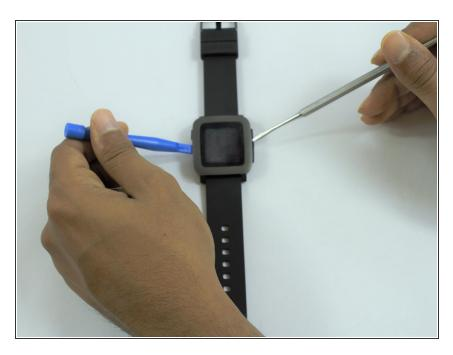
Use the metal spudger tool to carefully loosen the rest of the cover.
