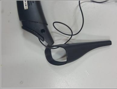
Gently remove the pointy rubber covering using tweezers where the speaker rests as shown in the picture.
