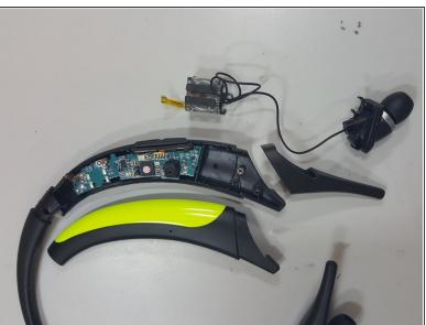
Desolder speaker connection using a soldering iron and replace with new speaker.
