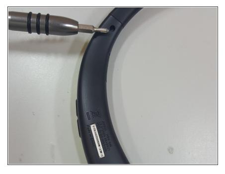
Remove hidden screw using a Philips #00 screwdriver.
