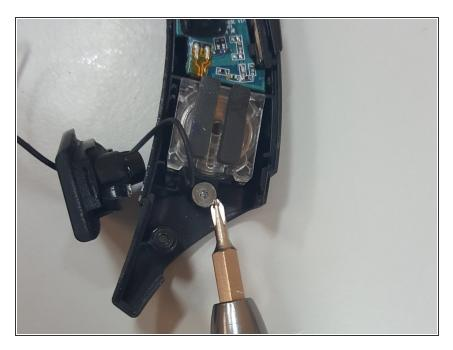
Remove the screw holding the speaker in place using a Philips #00 screwdriver.
