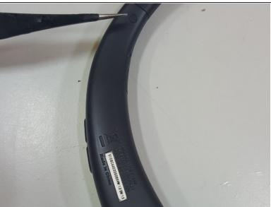
Locate the hidden screw as seen in the picture and remove the rubber covering the screw.
