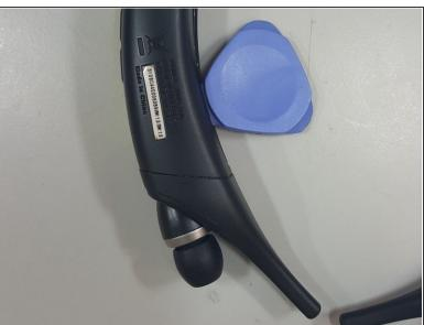
Use a guitar pick or any pry opening tool to gently lift the housing until the speaker end. There is a hidden screw that needs to be removed before the housing can be completely removed.
