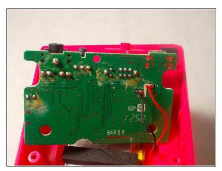
Remove the bad battery by unsoldering the red wire from the B+ solder joint and the black wire from the B-
