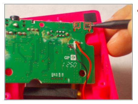
On the other side of the motherboard unsolder the two biggest solder joints under the micro USB.
