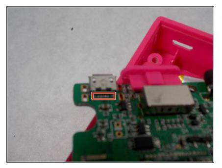
On the side of the motherboard that the micro USB connector is there are five surface mount solder joints at the back of the connector. Unsolder these five solder joints.
