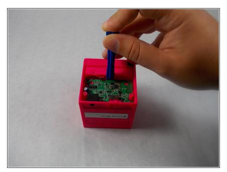
Take the motherboard out of the device, use the plastic opening tool to ensure the power switch doesn't get stuck.
