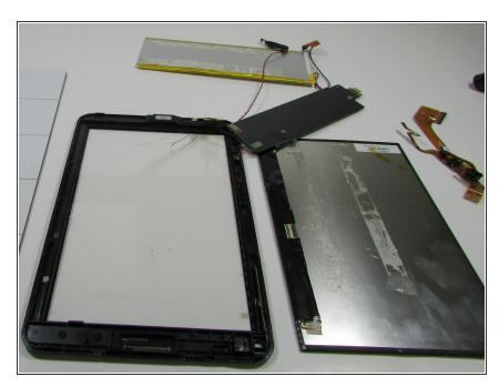
The touch screen should lift right out of the device.
