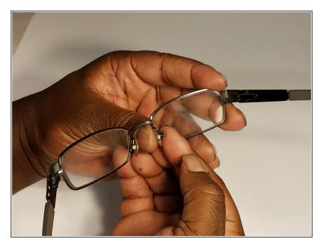
Unscrew the nose pad screw using a Phillips-head screw driver. Turn the screw counter-clockwise until the screw can be removed
