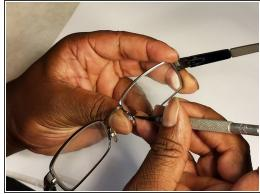
Remove the old nose pad and replace with a new one.
