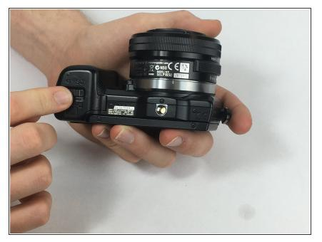
• Open the battery compartment by sliding the lock to the right.
