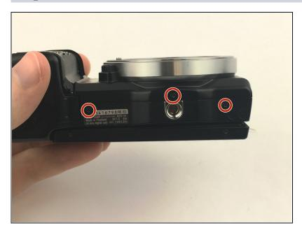
• Remove the 3.5 mm bottom screws.
