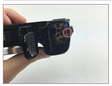
Remove the 3.5 mm bottom screw from the battery compartment.
