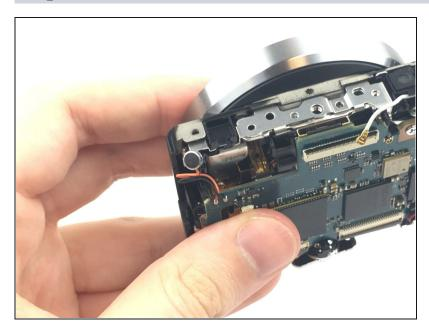
Pull the lead that was under the grommet out from the frame.
