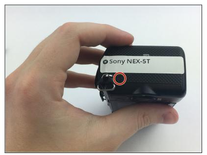
• Remove the 3.5 mm exterior-side screw.
