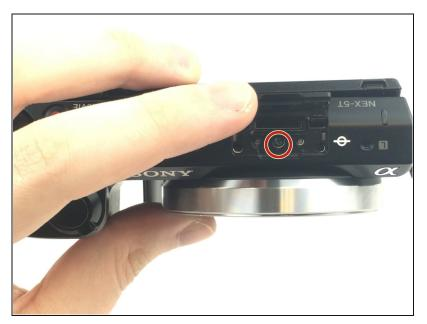
• Remove the 3.5 mm top flash-mount screw.
