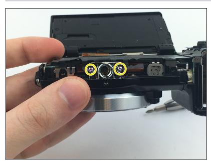
• Remove the 2.25 mm tripod mount screws.
