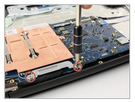
Using a Phillips #0 screwdriver, remove the two 3mm Phillips head screws from the metal bracket that covers where the wrapped cable from the screen attaches to the motherboard.
