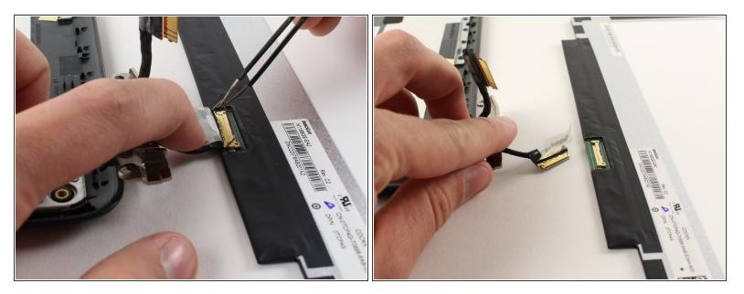
• To unplug the screen, use tweezers to lift the small metal wire on the connector, and then gently pull the cable away from the screen.
