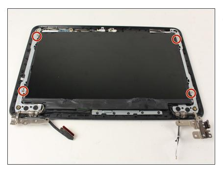
Using a Phillips #0 screwdriver, remove all four silver 3mm Phillips head screws that hold the screen tabs to the bracket.
