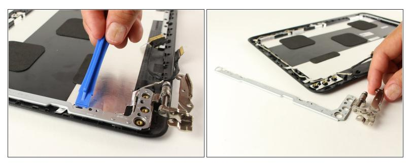
Once the screws have been removed, use a plastic opening tool to pry the metal bracket and hinge assembly off of the plastic backing.
