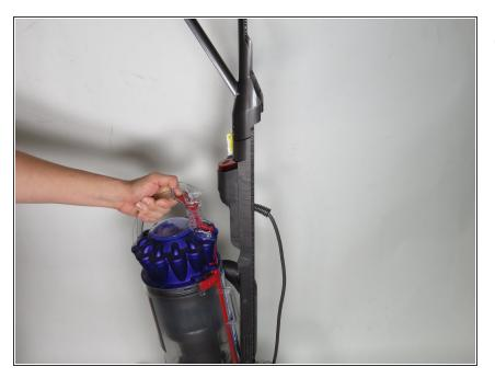
Remove the main canister by pressing the red release button and pulling up and away.
