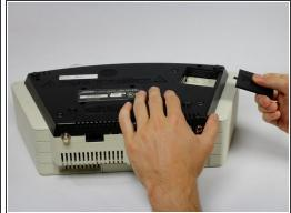
• Remove the battery cover by applying pressure and pulling away from the device.
