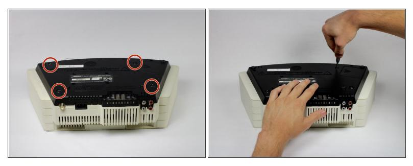
• Remove the four 19mm Phillips #2 screws from the base of the device.
