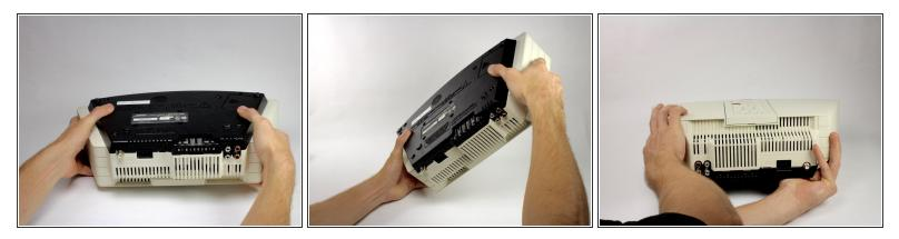
• Turn the device over, holding the base on with your thumbs.
