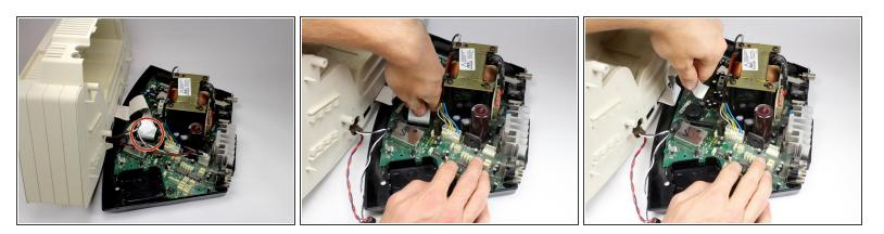
• Gently pinch and pull on the white ribbon cable to disconnect it from the base.
