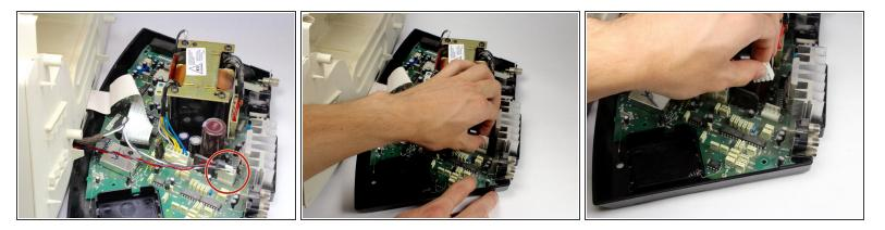
• Pinch and unplug the white connector from the device.
