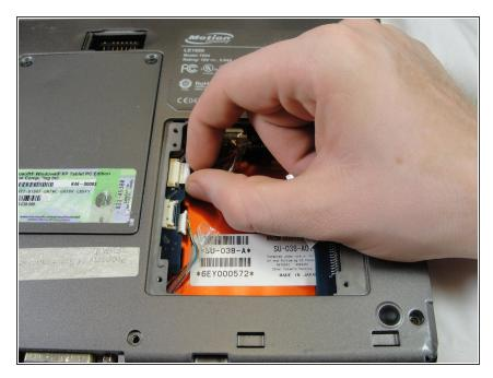
Pull the brown tabs to disconnect the white ribbon cable on the other side.
