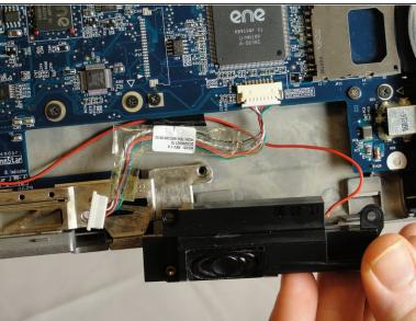
To remove the speaker near the headphone jack, unscrew the one 4mm black screw securing it to the tablet.
