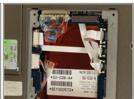
Pull clear plastic tab to detach hard drive from tablet.
