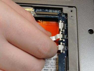
To disconnect the three white ribbon cables on the side closest to the hard drive connector, pull the white plastic tabs.
