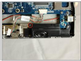
Locate speaker connectors on tablet and unplug them by pulling on the plastic heads.
