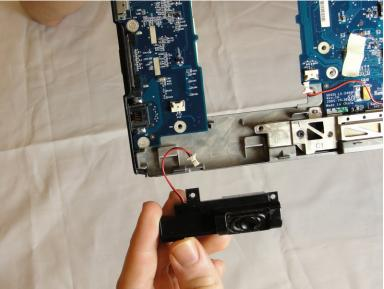
To remove the speaker near the network port, unscrew the two black 4mm screws securing it to the tablet and pull away.
