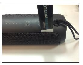
Using a pry opening tool, pry into the speaker grill covering as seen in the photos.
