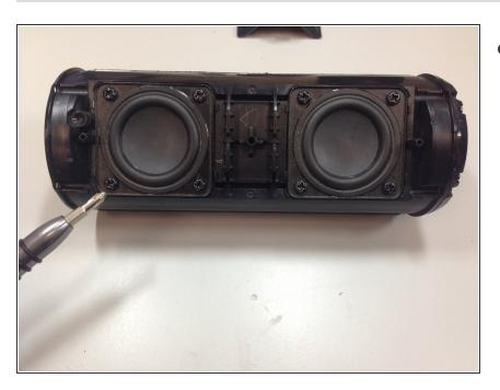
Remove all 8 speaker screws using a Philips 00 screwdriver.
