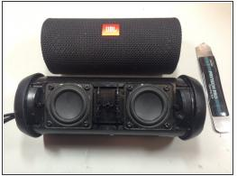
Continue to pry open the grill all the way around until it can be removed from the unit itself as seen in the pictures.
