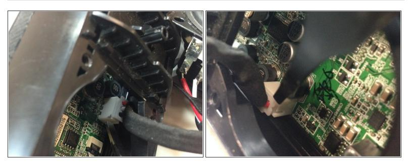
Using tweezers, carefully remove both side speakers from the motherboard as shown in the pictures.
