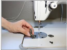
Use a screwdriver to disassemble the presser foot.
