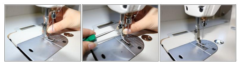
Use the screwdriver to assemble the new presser foot.
