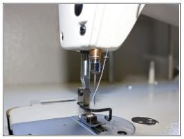
Roll the hand wheel on the right side of the machine to raise the needle up.
