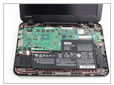
Lift the keyboard up and off the back panel, exposing the motherboard and battery.
