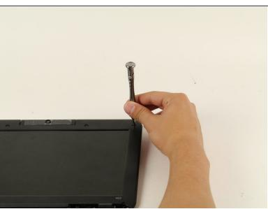
Use a Phillips #1 screwdriver to remove the six 4mm screws. Rotate the screws to the left with the screwdriver.
