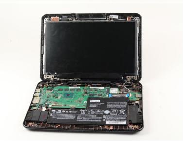
Remove the panel from the front casing by lifting any two corners.
