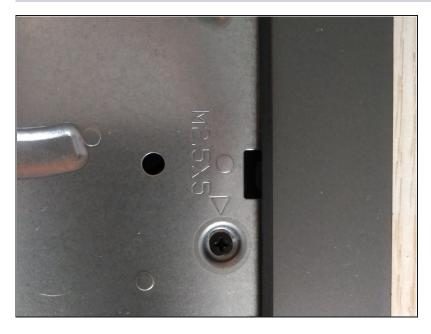
Remove the screw on the upper side of the laptop.
