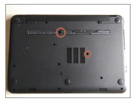
Remove the two indicated screws using a #1 Phillips driver.
