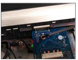
Remove the two screws holding the main board to the plate (see pictures two and three).
