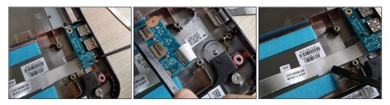
• Use a spudger to loosen the cable from the bottom plate.
