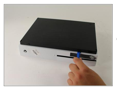
Begin by working at the case on the rear where the warranty sticker is located. Insert the plastic opening tool into the gap between the bottom of the case and the grated top side. Then find the clips in between that hold the case in place. Use the opening tool to pop the clips out. The best method is to pry the black case away from the bottom.
