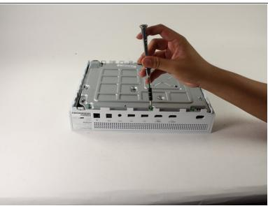
Use a T10 Torx screwdriver to remove the six green 50 mm long screws from the metal case labeled F1 through F6.
