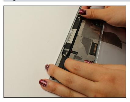
• Slide both speakers out from the edges of the device.
