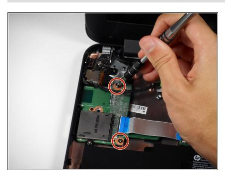
Remove the two Phillips #00 6mm screws that attach the module to the laptop.
