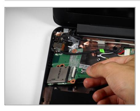
Lift the module up and out of the laptop.
