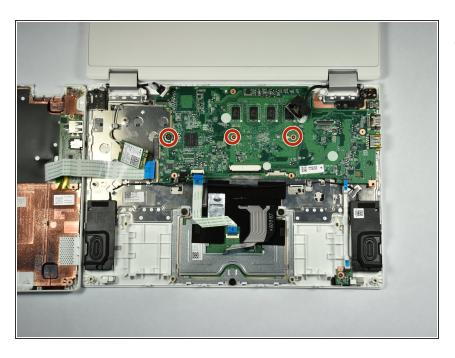
Remove the two 4.5 mm screws and a 2.0 mm screw from the middle of the motherboard.
