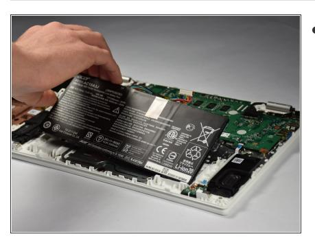
Lift the battery out by pulling upward.
