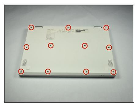
Using a Phillips screwdriver, remove all eleven 7.0 mm screws from the bottom of the Chromebook.
