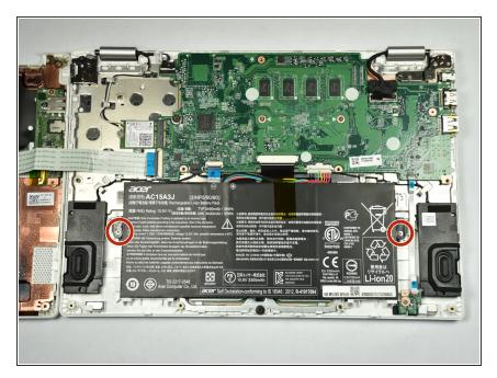
Remove the two 4.5 mm Phillips screws located at the sides of the battery.
