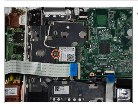
Remove the 2.0 mm screw from the Wi-Fi card.
