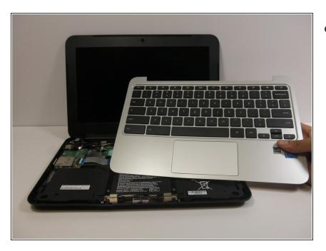
Remove the keyboard assembly by lifting it off the laptop base.
