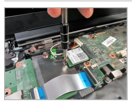
Remove the 4 mm Phillips #1 screw on the Wi-Fi card.
