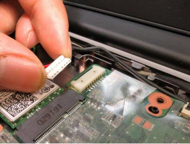
Remove the cable at the top left of the motherboard by grabbing the male connector and applying force in the direction of the wires away from the motherboard.
