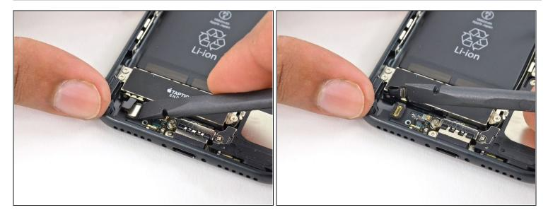
• Use the flat end of a spudger to disconnect the Taptic Engine connector from its socket on the logic board.
