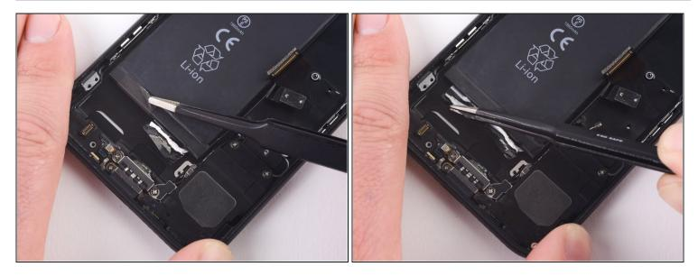
• Use a pair of tweezers with blunt tips to peel back the other adhesive strip on the lower edge of the battery.
