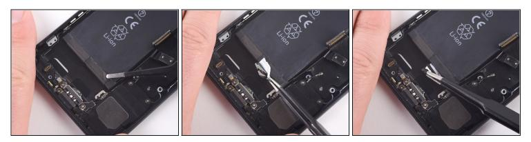
• Use a pair of tweezers with blunt tips to peel back one of the adhesive strips on the lower edge of the battery.
