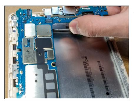
Remove the motherboard by pulling it straight up and away from the tablet body.
