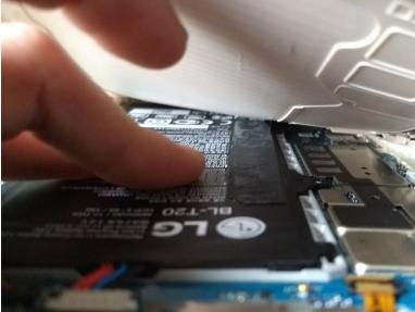
Gently pull the back cover away from the adhesive on the battery.
