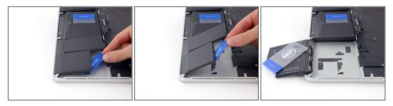
• Flip the two de-adhered right-hand battery cells over the front edge of the MacBook Pro, if you haven't already. This will allow access to the outside edge of the center cell.
