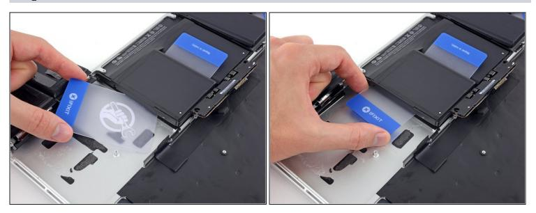
• Push one corner of a plastic card below the plastic battery frame and underneath the remaining adhered edge of the lower center cell.
