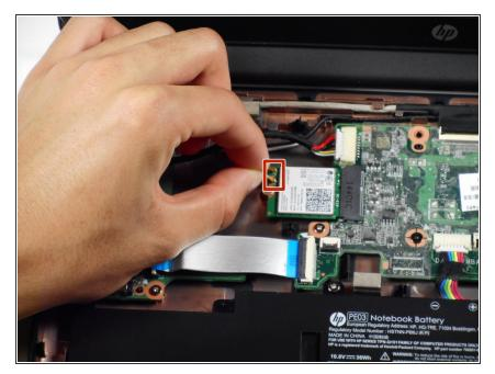
Gently tug on the black and white wires connected to the Wi-Fi module to disconnect them.
