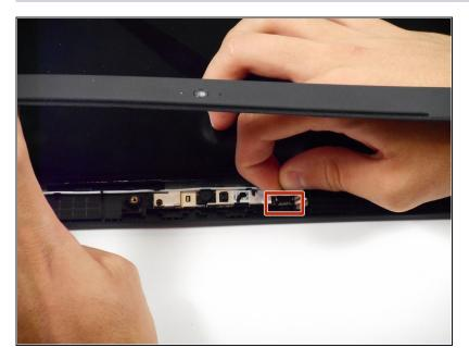
• Gently remove the slide-out connector near the bottom left corner of the camera mount.
