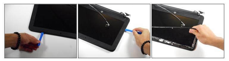
• Use the plastic opening tool to pry the left and right side of the top of the lid, and proceed inwards from the sides.
