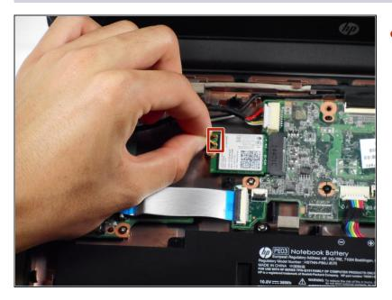
Gently tug on the black and white wires connected to the Wi-Fi module to disconnect them.
