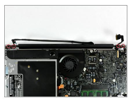
Remove the two outer 6 mm Torx screws securing each side of the display to the upper case (4 screws total).
