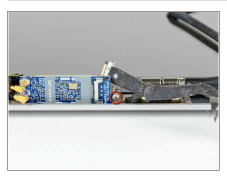
Remove the remaining 3 mm Phillips screw securing the side of the AirPort card closest to the right clutch hinge.
