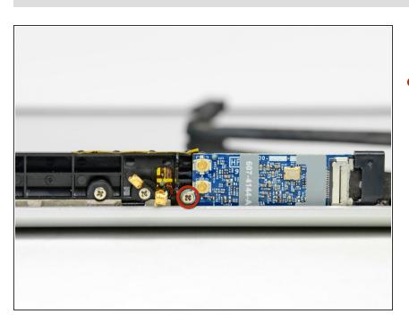
Remove the single 3 mm Phillips screw securing the AirPort card to the display nearest the AirPort antenna.
