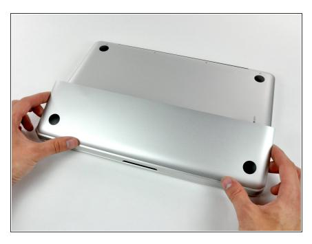
The access door should now be raised enough to lift it up and out of the Unibody.
