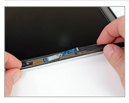
Use the flat end of spudger to flip up the Bluetooth board from its recess within the display assembly.
