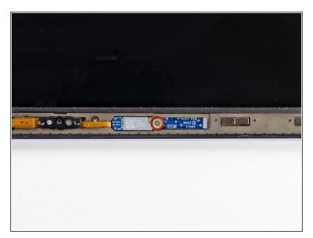
Remove the single 3 mm Phillips #00 screw securing the Bluetooth board to the display assembly.
