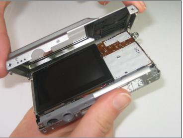
With the LCD screen facing up towards you, start at the bottom of the camera and gently pull off the back of the casing.
