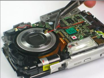
• Use a pair of <u>tweezers</u> to gently move the wire around part of the lens away from it so that you can access the lens.
