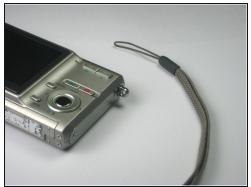
• Remove the strap from the camera by pulling the thin cord out, creating a small loop, then pushing the thicker cord back through this loop.
