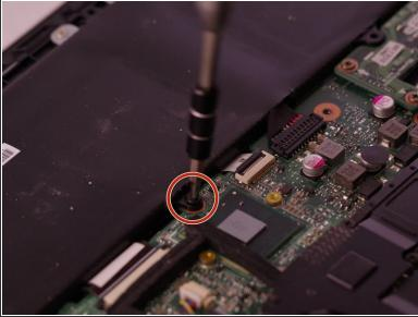
Using the same Phillips #0 screwdriver, remove the eight black 50mm screws surrounding the battery.
