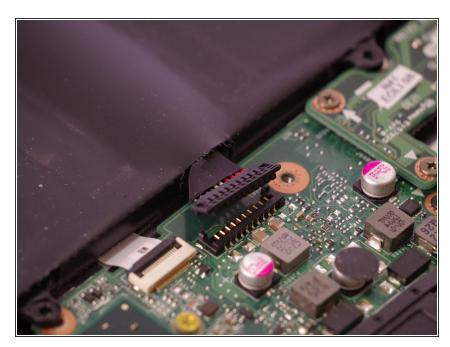
Using a set of precision tweezers, lift the motherboard connector tab.
