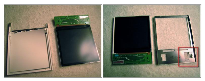
• The screen is sandwiched in a metal case. It didn't seem clipped together but it was a snug fit. I pushed on the circuit board through the cutouts in the metal to pry the pieces apart.
