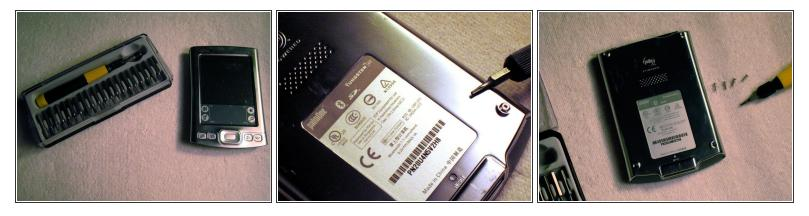
There are four T6 screws on the backside of the Palm which must be removed for access into the inner workings. The tool is a T6 screwdriver, available in the parts store. Either purchased separately as the <u>T6 Torx screwdriver</u> or as a kit in the 20 Piece Bit Driver Kit.
