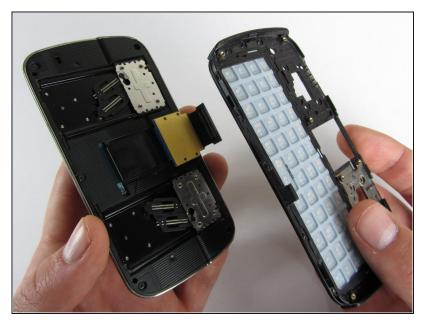
• Carefully remove keyboard frame from the sliding mechanisms underneath.
