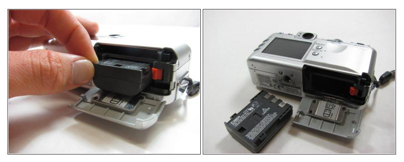
• Holding the edges, slide out the battery.
