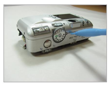
• Using a spudger, gently separate the back panel from the rest of the camera and remove it.
