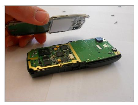
Once the six screws are removed, you may take off the screen section of the phone, exposing the inner workings of the cell phone.
