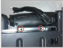
You should be left with this. From here you will need to remove the 4 bolts on the upper part of the footrest: 2 on the right, and 2 on the left. From here the top should separate from the metal piece.
