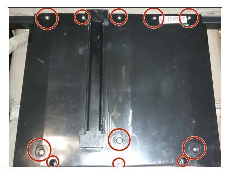
• Before starting this step you will need to remove the footrest from the chair. This is done by removing the 5 screws at the top and the 6 screws at the bottom. The plastic shroud will come off as one piece, however it has 2 pieces that slide into each other.
