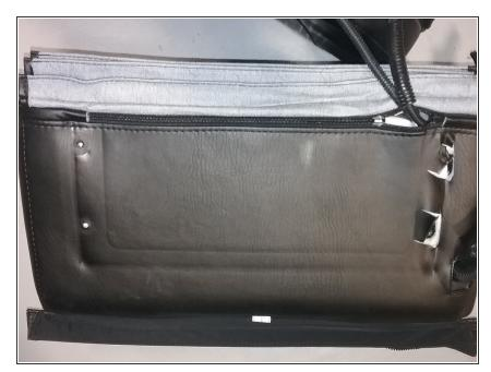
Once separated be careful because the top is connected to the bottom by an air hose and wire. The top is zipped to the bottom. Please unzip before continuing to next step.
