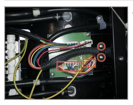
Remove the back cover and this is what you are left with. Remove the 2 screws and that will free up the wire harness. Unplug the cable from the board and attach new cable. Upon re installation you will need spray adhesive.
