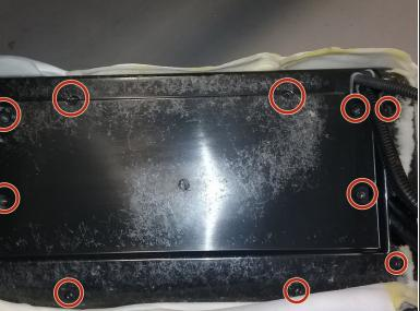
Next step is to unzip the leather from the bottom piece. Once unzipped you should be left with this. From here, just carefully pull back the foam to reveal the back cover and screws. Remove the back cover by unscrewing the 12 screws. Unfortunately, due to photo size limitations I'm unable to show all 12.
