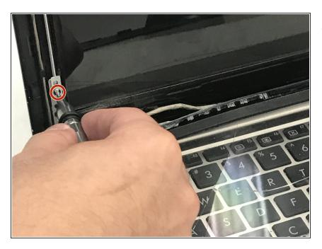
Remove the two 2.8 screws on the bottom right and left using a Phillips #0 screwdriver.
