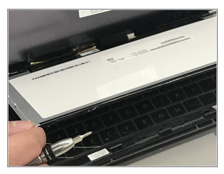
Once the screws are removed you should be able to move the display down. Be careful as there is a connection to the motherboard which will need to be removed.
