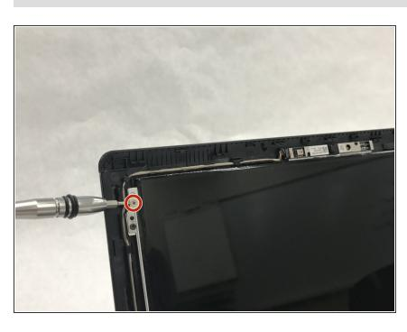
Remove the two 2.8mm screws on the top right and top left of the screen using a Phillips #0 screwdriver.
