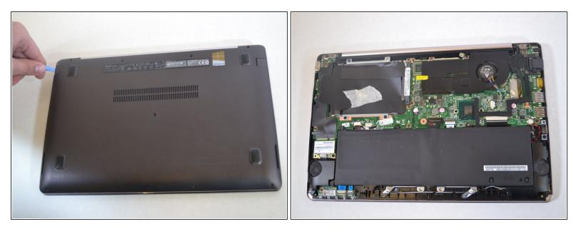
• Use a plastic opening tool to gently remove the back panel.
