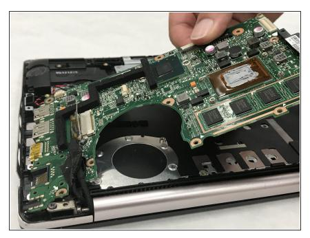
• Carefully lift the motherboard up out of the slot.
