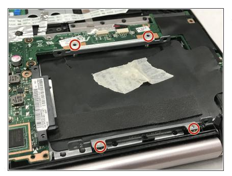
Unscrew the four 5.9mm hard drive bracket screws with a Phillips #0 screwdriver.
