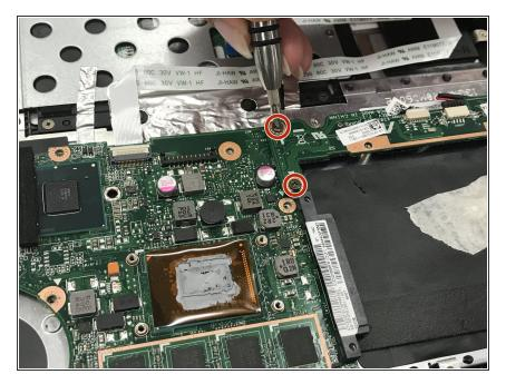
Unscrew the two 5.9mm screws on the PCB board with a Phillips #0 screwdriver.
