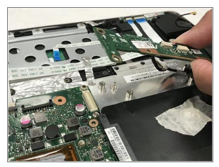
• Remove the PCB board from the motherboard.
