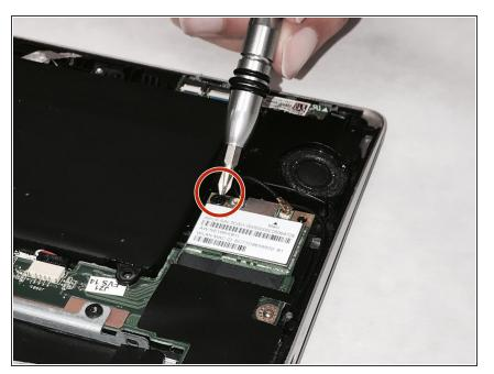
Remove the one 4.9mm screw that holds the wireless card in place with a Phillips #00 screwdriver.
