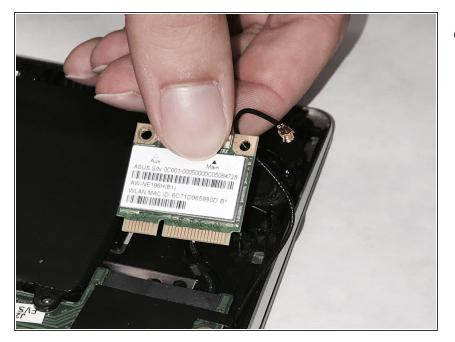
• Pull the wireless card from connector slot.
