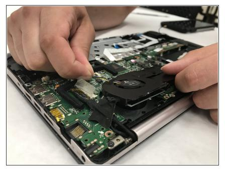
• Lift up and remove the cooling fan from the slot.
