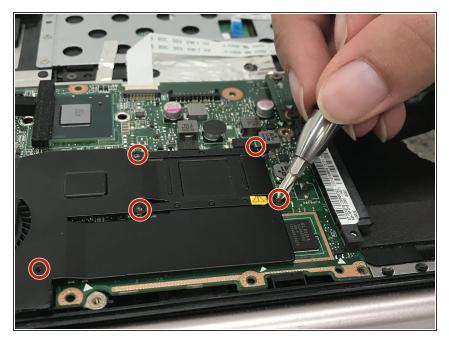
• Unscrew the five 4.9mm screws holding the cooling fan in place using a Phillips #0 screwdriver.
