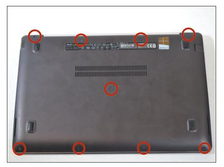
Remove the nine Philips #00 screws holding the back panel in place (four 5.6mm, four 7.7mm, and one 9.2mm).
