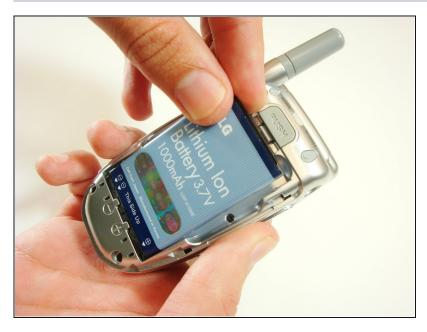
• Lift up on the battery to remove it from the case.
